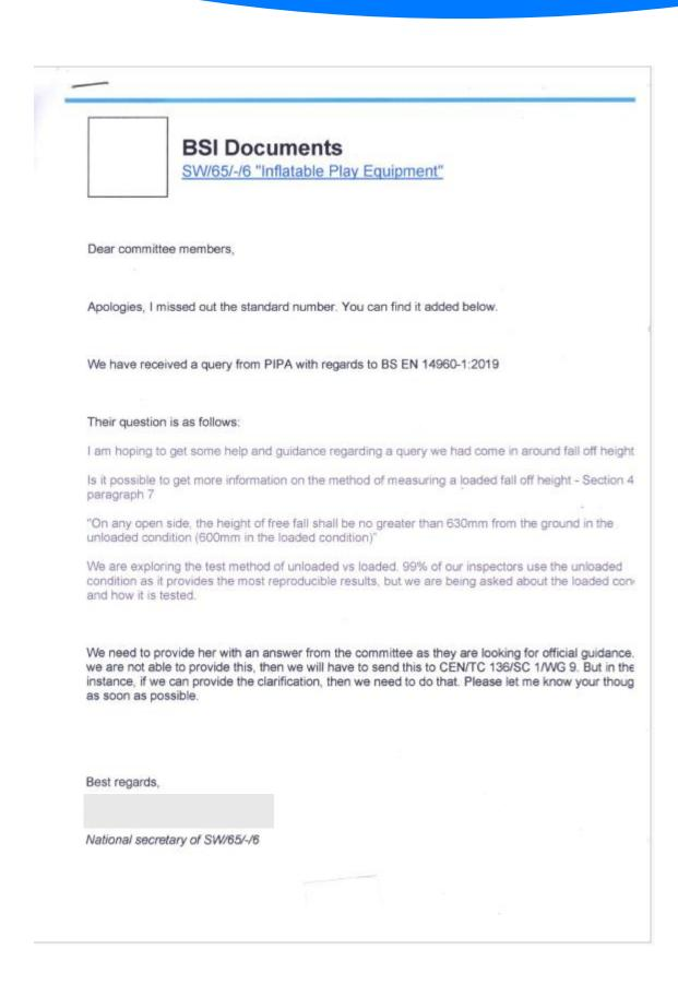
On any open side the free height of fall shall be no greater than 630 mm from the ground in the unloaded condition.
